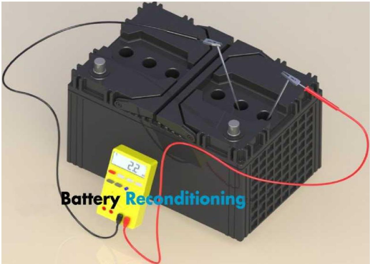
This process must be repeated by moving down the row of cells until the voltage of all the cells has been checked. You must get a reading of at least 2 volts for
