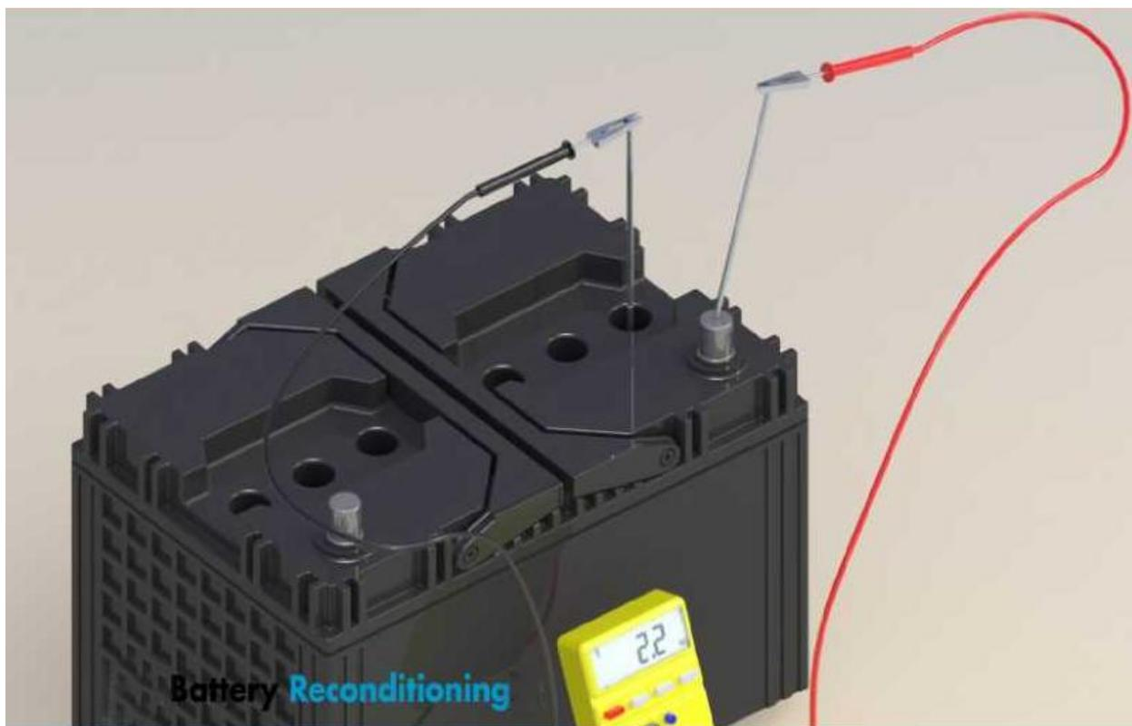
**Testing the 2<sup>nd</sup> Cell (and on):** Next, to check the second cell, connect the red probe to a wire and place it in the first cell and connect the black probe to a wire and place the wire in the second cell. You should again get 2 volts.
