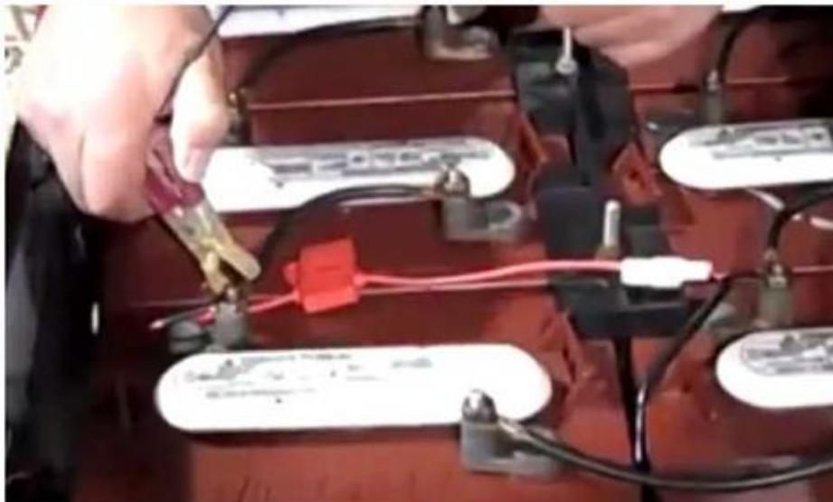
Make sure that you unplug the car battery charger every time you connect and disconnect the clamps to the corresponding battery terminals to avoid this.
