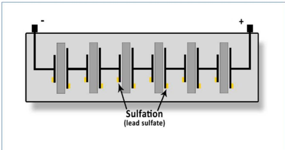
**Description:** Schematic diagram of the inside of a 12v battery that is fully charged (with minimal sulfation on the plates).
