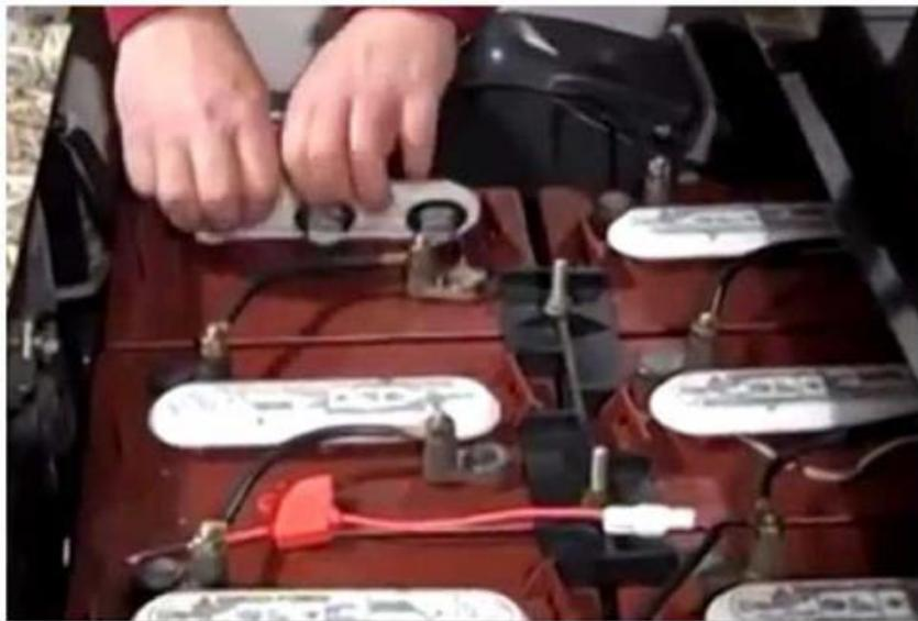
**Step 3:** Take a regular, 12 Volt, wall-plugged car battery charger, hook up the positive clamp to the positive terminal on the first battery in the series, and take the negative clamp and hook it up to the negative terminal of the second battery.
