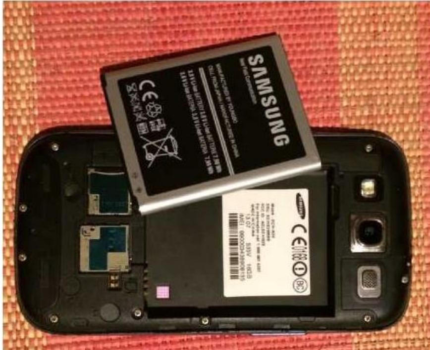
**Step 3:** Locate the polarity markings on your phone battery.
