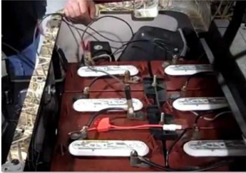
**Step 2:** Open up the battery and check if there is enough water covering all of the plates in each cell. If not, add distilled water as needed.
