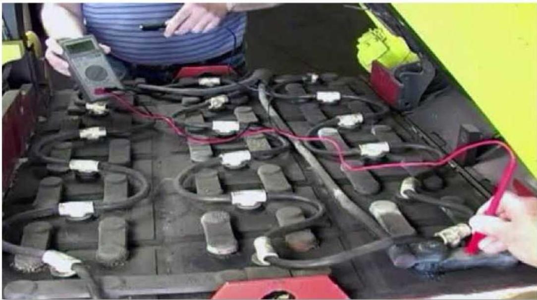
This reading should be about equal to the operating/rated voltage of the battery. It's even possible for it to be a little higher if the battery was just charged. But if the overall voltage is lower than the rated voltage, then the battery has some cells that are weak.
