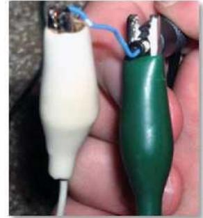
You can then use a little bit of wire and put it into the center of the middle hole and use that to connect the positive of the charger to the positive terminal of the battery with an alligator clip (to hold it in place).
