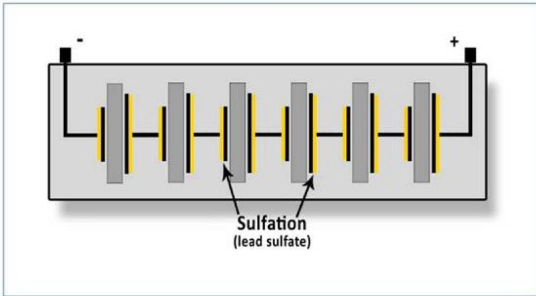
**Description:** Schematic diagram of the inside of a 12V battery that is discharged down to 10.5V
