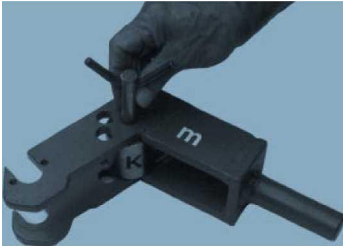
To start bending we use a bending-claw m with accessory cylinder K plus half-shaft. Put cylinder K half-shaft into the third hole of bending-claw m.
