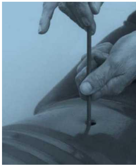
Debur the holes with a round file until the holes have diameter of 18 mm
