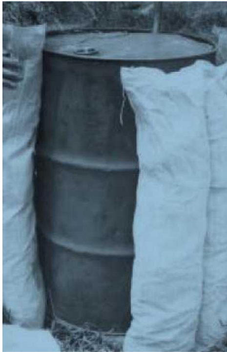
The total width of the self-made covers must easily surround the circumference of the drum
